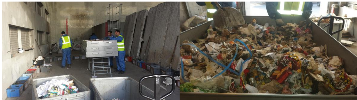
Figure 9. Tri de la fraction > 100 mm.
